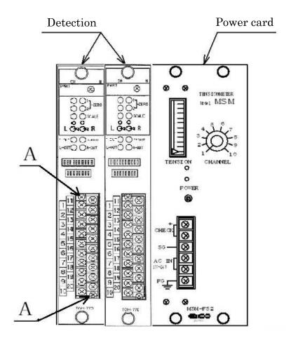
(3) To remove a card, pull the knobs on the top and bottom of each card toward you. To install the card, insert the card firmly and push the knob in to lock it in place. Please turn off the power before inserting or removing the card.
