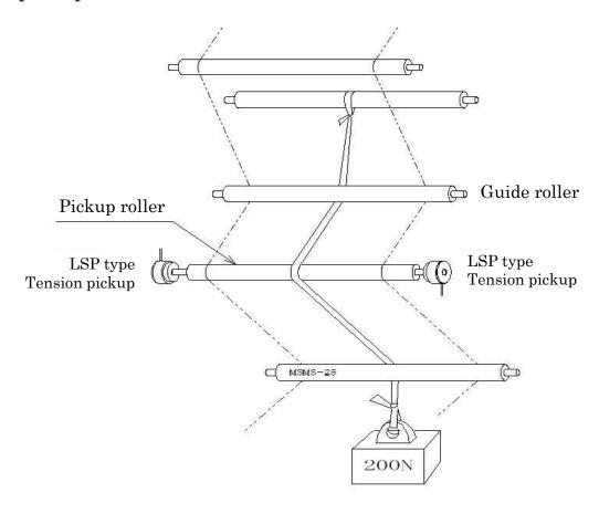
②Single pickup: A configuration in which a pickup is attached to one side of the pickup roller.
