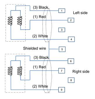
Use three-core shielded wires for the connections to LA-type tension detectors, and connect the shielded area to the terminal No. 5.
